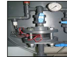
Novel Electro-Fenton filter
