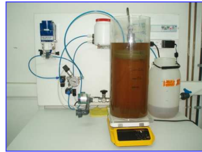
Schematic diagram and a view of lab-scale pilot unit for pre-treatment (clarification by UF membranes) of agro-industrial wastewaters containing high-added value substances
