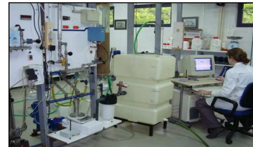
Pilot unit for continuous monitoring of scaling potential in desalination plants.
