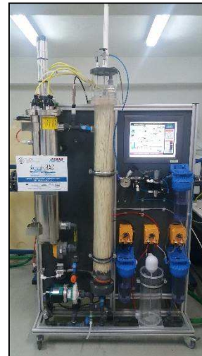
PMR Pilot plant; continuous, unattended, remotely monitored operation
